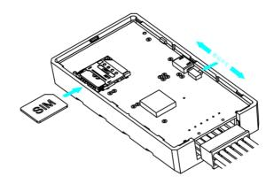
Assembly the SIM card and turn on the switch
